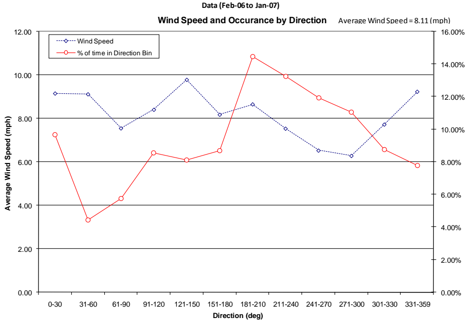
Figure E.7.7. Average wind speed for each direction bin and % time in that bin.
